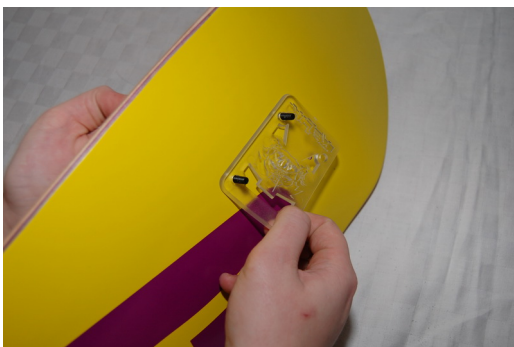
fig 31: Attach a riser pad to the truck mount bolts
