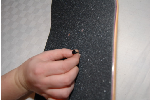
fig 30: From above, extend the truck mounting screws through the pre-drilled holes in the deck
