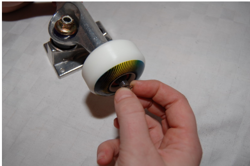
fig 27: Attach the second speed ring to the truck
