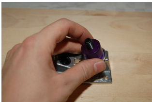
fig. 15: Attach the larger of the two bushings to the kingpin
