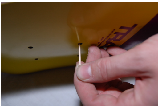
fig 21: Pierce the griptape to mark the pre-drilled holes.
