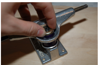
fig. 18 Attach the smaller of the two washers kingpin on.
