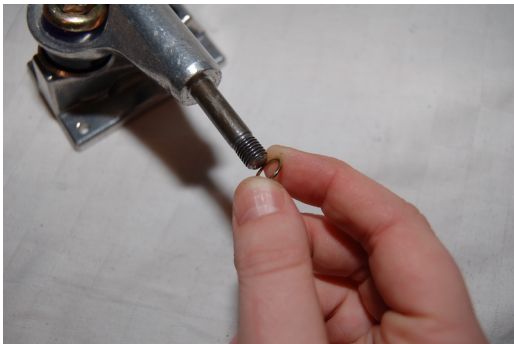
fig 25: Attach a speed ring to the truck
