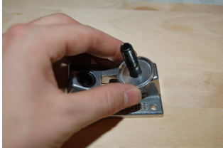
fig. 14: Attach the larger of the two washers to the kingpin
