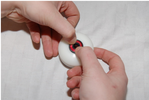
fig 24: Push the second ball bearing into the wheel
