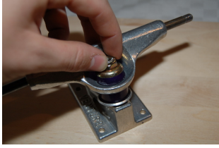
fig. 19: Attach the hangers and rubbers with the kingpin nut
