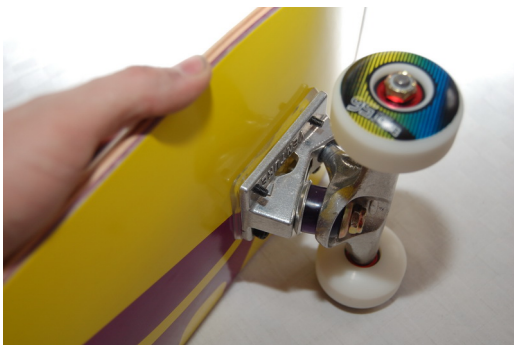
fig 32: Attach a truck to the truck mounting bolts
