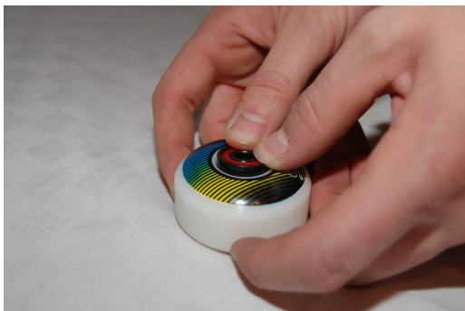
fig 22: Push a ball bearing into the wheel
