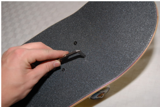
fig 35: Make sure the truck mounting screws do not protrude
